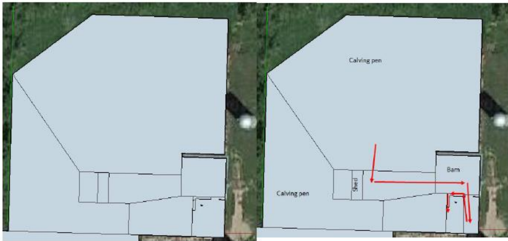
Figure 2: Pens of main working facility; current flow of cattle through the facility shown in red.
